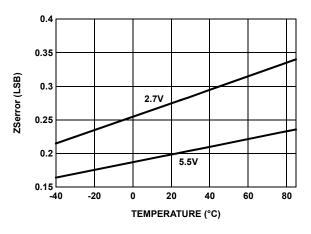
FIGURE 5. ZSerror vs TEMPERATURE FOR 50k $\Omega$  (W)
