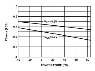
FIGURE 6. FSerror vs TEMPERATURE FOR 50k $\Omega$  (W)
