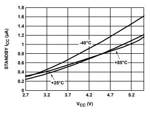
FIGURE 2. STANDBY ICC vs VCC
